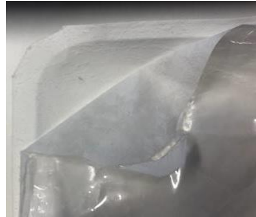
Separation plastic laminated film from cardboard (ex. 1)
