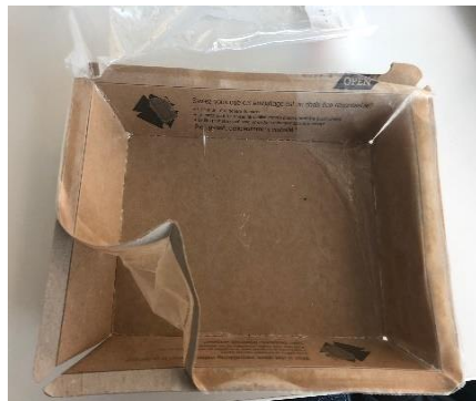
Separation plastic laminated film from cardboard (ex. 2)
