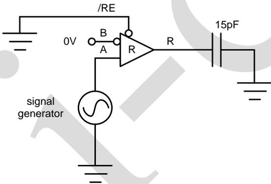
Figure 5A. test circuit
