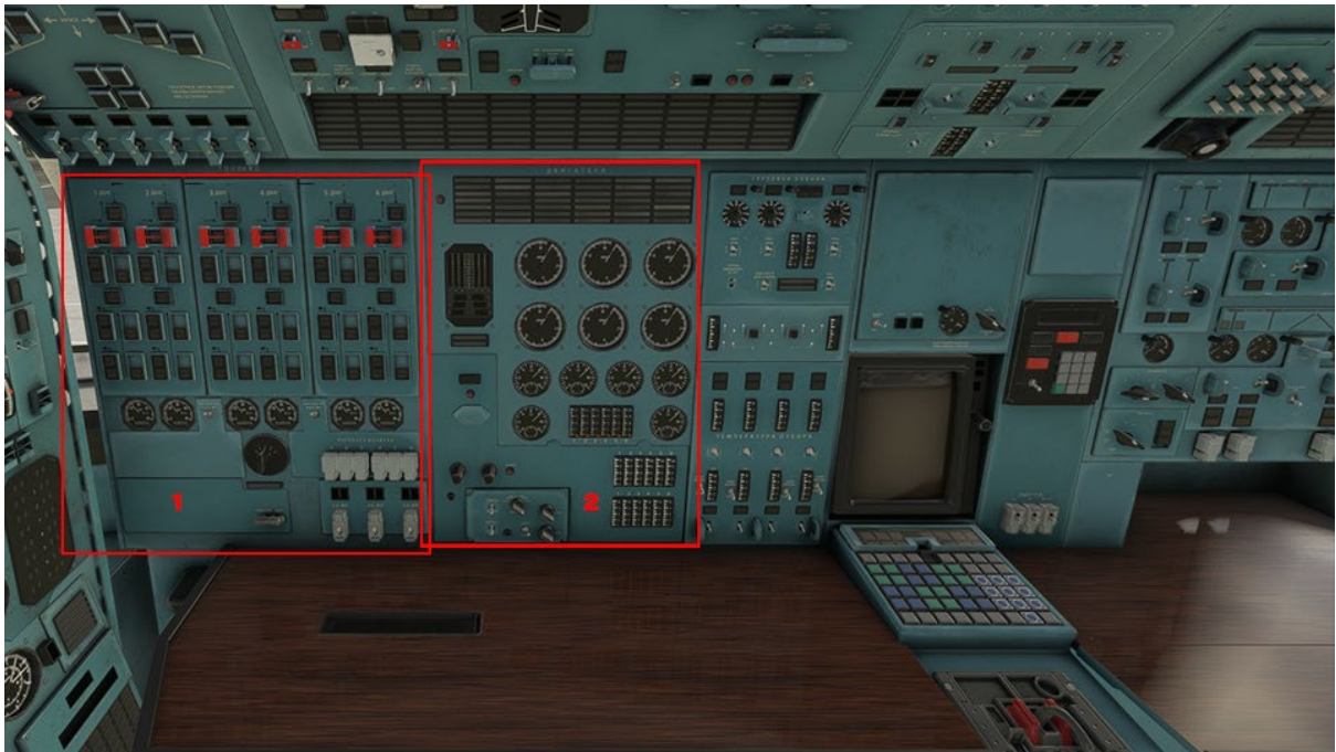
1. Fuel Panel (FO Side)
