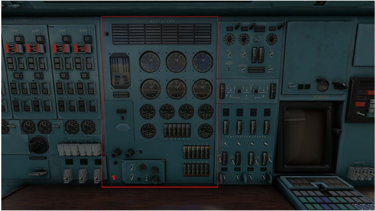
1. Engine Panel (FO Side)
