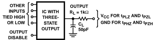
NOTE: Open drain waveforms  $t_{PLZ}$  and  $t_{PZL}$  are the same as those for three-state shown on the left. The test circuit is Output  $R_L = 1k\Omega$  to  $V_{CC}$ ,  $C_L = 50pF$ .
