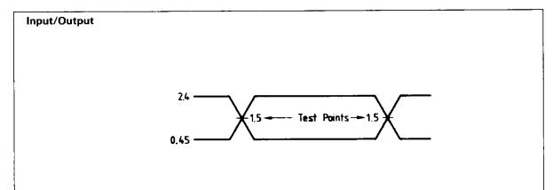
A.C. Testing Inputs are driven at 2.4V for a logic "1" and 0.45V for a logic "0". The clock is driven at 4.3V and 0.25V timing measurements are made at 1.5V for both a logic "1" and "0"  $^{\prime\prime}$ ".
