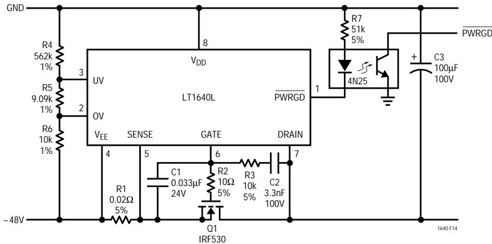
Figure 14. Using  $\overline{\text{PWRGD}}$  to Drive an Optoisolator
