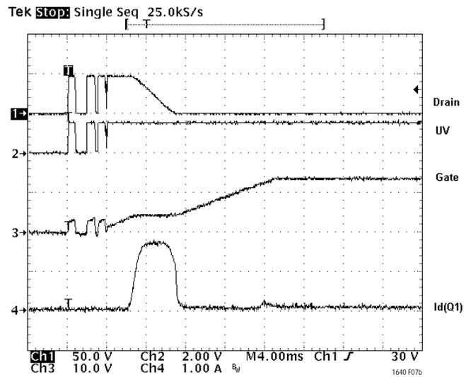
Figure 7b. Improved Inrush Control Waveforms
