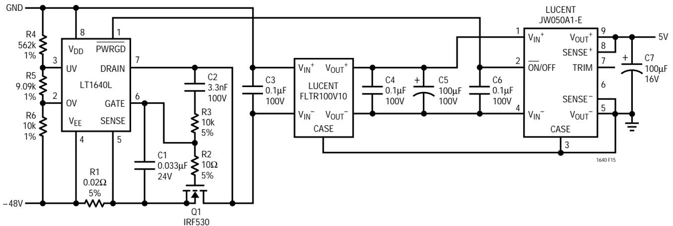
Figure 15. Typical Application Using a Filter Module
