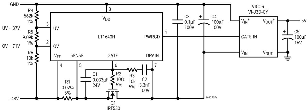
Figure 7a. Improved Inrush Control Circuitry
