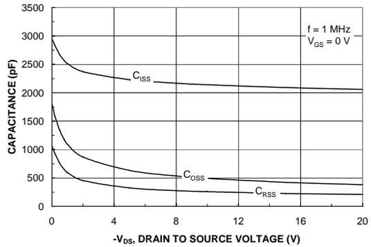
Figure 8. Capacitance Characteristics.
