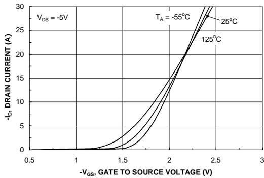
Figure 5. Transfer Characteristics.
