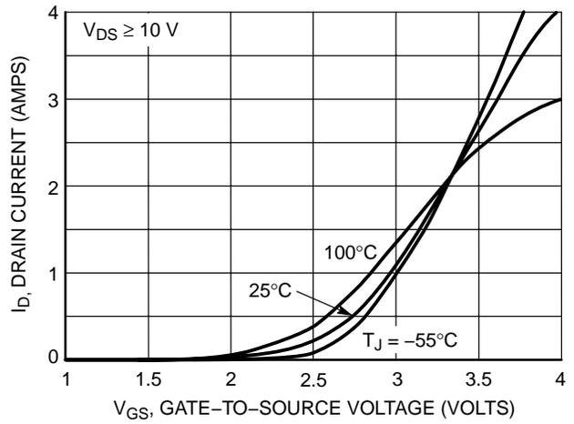
Figure 2. Transfer Characteristics
