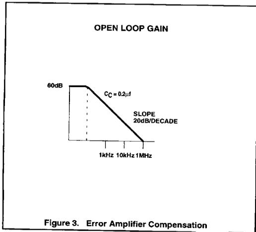
Figure 3. Error Amplifier Compensation
