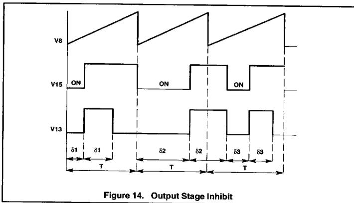
Figure 14. Output Stage Inhibit
