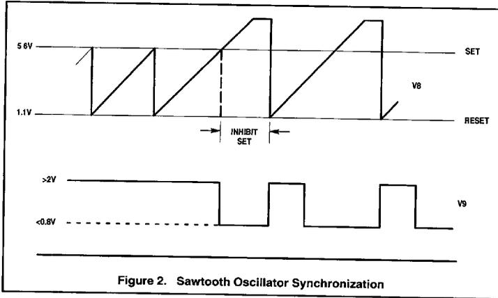
Figure 2. Sawtooth Oscillator Synchronization
