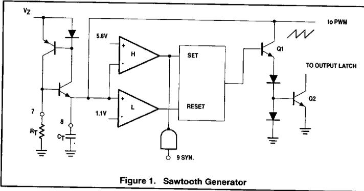
Figure 1. Sawtooth Generator
