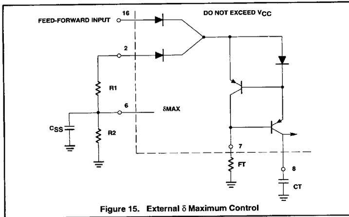
Figure 15. External  $\delta$  Maximum Control
