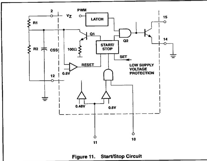
Figure 11. Start/Stop Circuit
