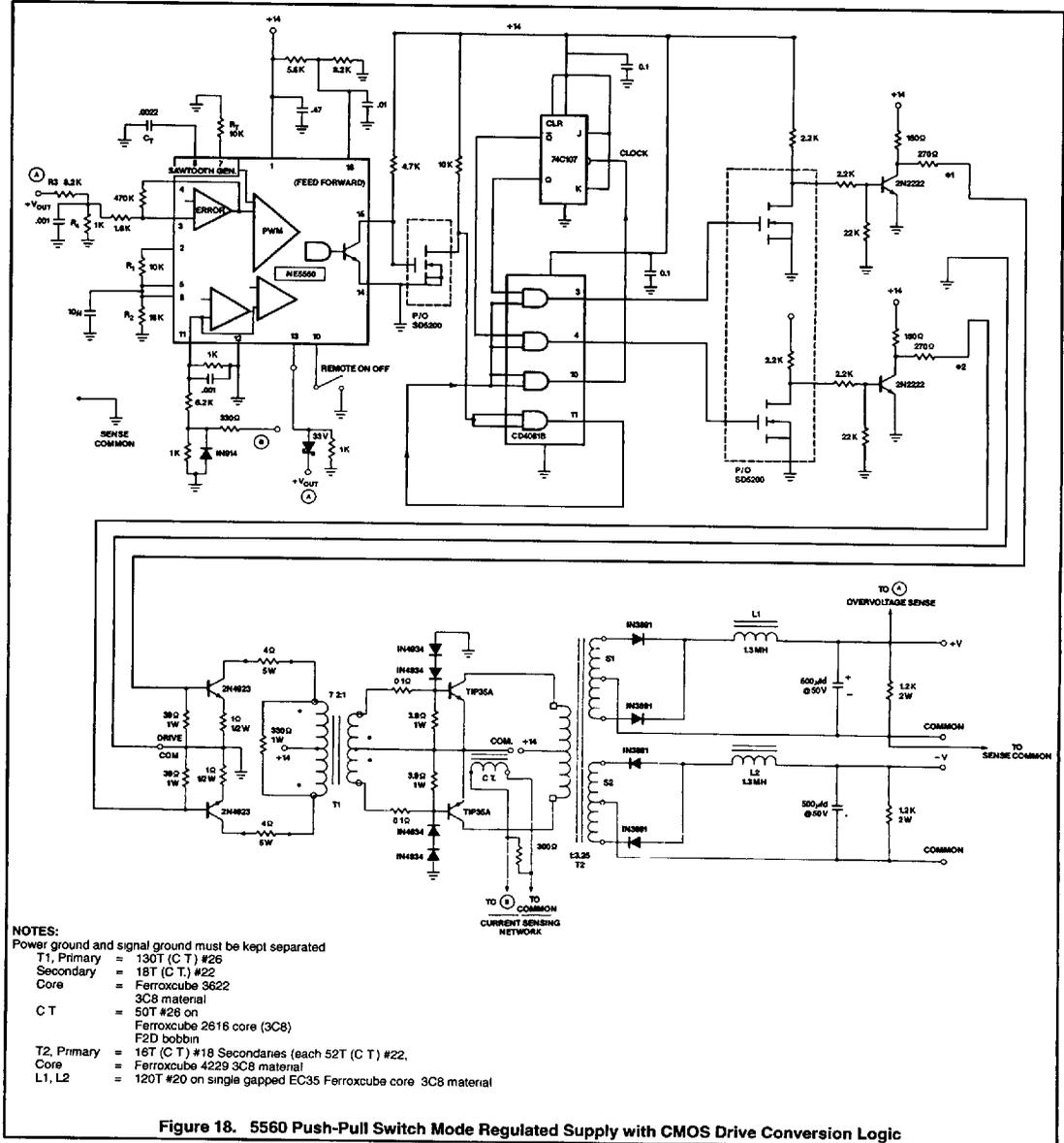
Figure 18. 5560 Push-Pull Switch Mode Regulated Supply with CMOS Drive Conversion Logic
